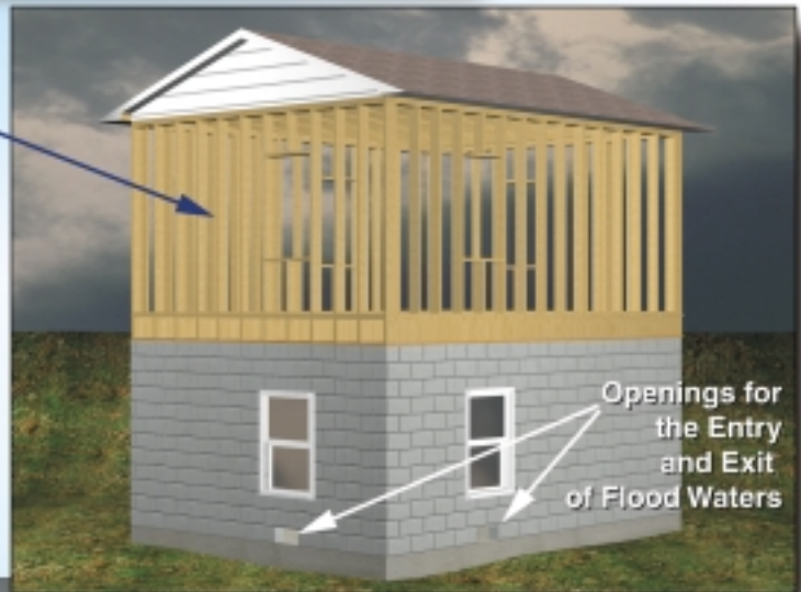
Substantially damaged house undergoing repairs that will bring it into compliance with Miami-Dade County floodplain management requirements
